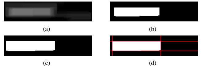
Fig. 3. Operations in a candidate regarding the vehicle license plate: (a) Region corresponding to the image obtained at the end of Section II-B; (b) Region binarization; (c) Erosion and dilation; (d) Bounding box update.
