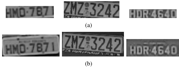
Fig. 4. Examples of labeling of images: (a) Minimum bounding box that includes all the characters; (b) Minimum bounding box that includes the entire vehicle license plate.
