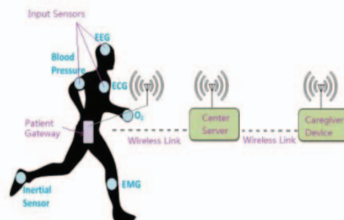
Fig. 1. The patient health data monitoring system used in this study
