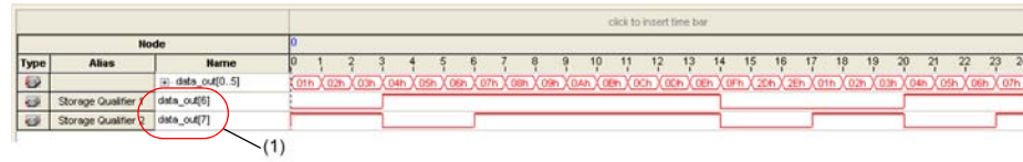
Figure 15-20. Data Acquisition of a Recurring Data Pattern in Continuous Capture Mode (to illustrate Conditional capture)
