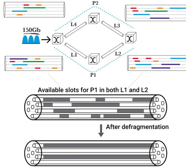
Fig. 1. EON-SDM optical network with high fragmentation.
