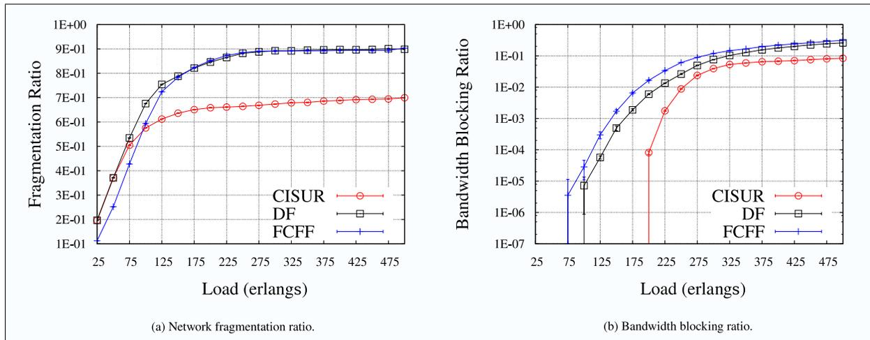
Fig. 4. Results extracted from the NSFNET topology; charts on the left side give the fragmentation ratio whereas those on the right side give the BBR.
