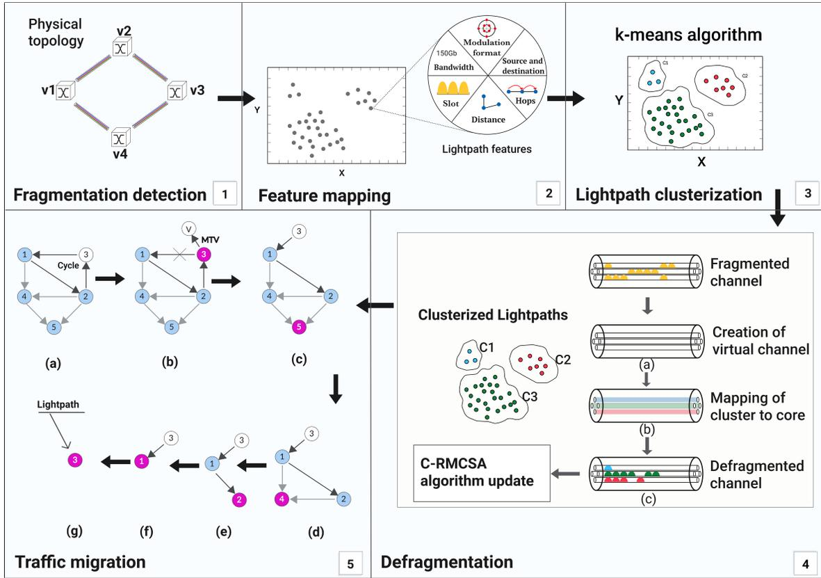
Fig. 2. Defragmentation flowchart in SDM networks using unsupervised learning. The CISUR algorithm is divided in the following steps: (1) verification of the need for defragmentation, (2) features mapping, (3) clusterization of lightpaths, (4) rearrangement, and (5) traffic migration.
