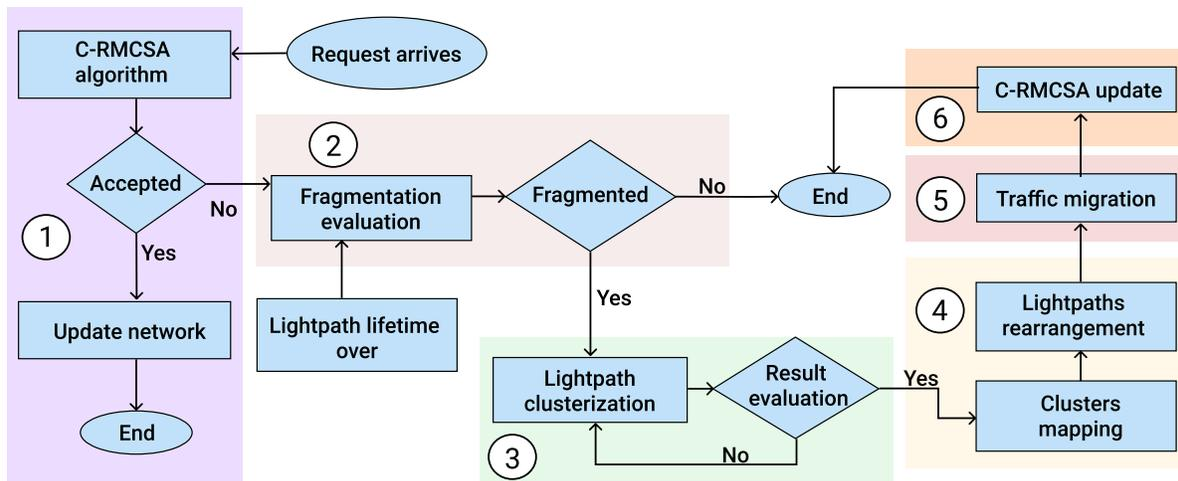
Fig. 3. Illustration of how the CISUR and C-RMCSA algorithms are integrated.
