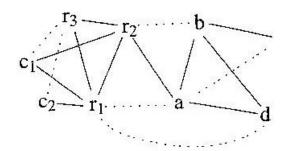
9. Graph-coloring proceeds as follows. We  $r_3c_1c_2$  can immediately coalesce  $c_1\&r_3$  and then  $c_2\&r_3$ .
