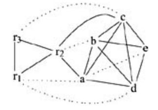
Node c has the lowest priority – it interferes r<sub>3</sub> with many other temporaries but is rarely used – so it should be spilled first. Spilling c, we obtain the graph at right.
