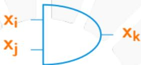
$$\begin{aligned} & x_i \wedge x_j \Leftrightarrow x_k \\ \equiv & (\neg x_i \vee \neg x_j \vee x_k) \wedge (x_i \vee \neg x_k) \wedge (x_j \vee \neg x_k) \end{aligned}$$
