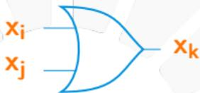
$$\begin{aligned} & x_i \vee x_j \Leftrightarrow x_k \\ \equiv & (x_i \vee x_j \vee \neg x_k) \wedge (\neg x_i \vee x_k) \wedge (\neg x_j \vee x_k) \end{aligned}$$
