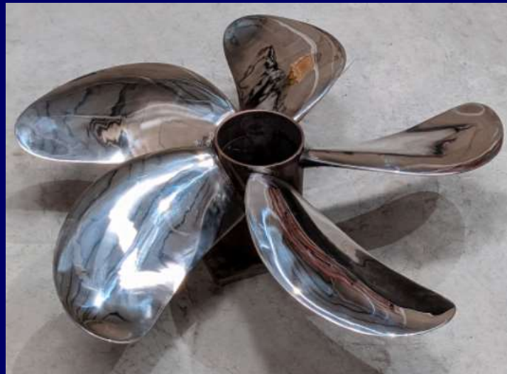
SS316L – Naval Propeller Size: 600 Ø mm Weight: 12,1 kg Print Time: 43 h 40 min
