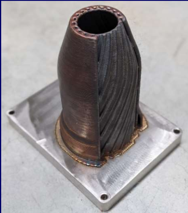
SS316L – Combustion Chamber Size: 110,5 x 110,5 x 170 mm Weight: 4,88 kg Print Time: 27 h 30 min
