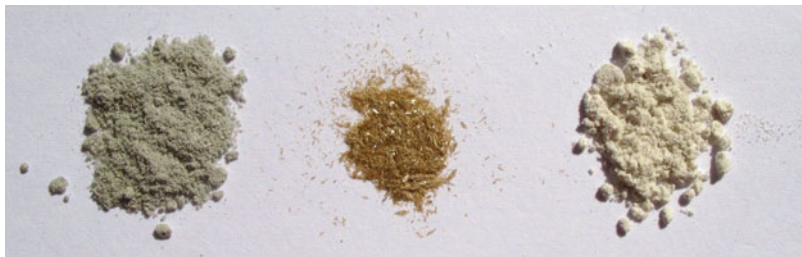
Fig. 3.1 The three common forms of mercury fulminate from left to right —gray, brown, and white
