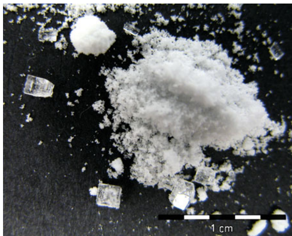
Fig. 10.7 Spontaneous recrystallization of powdery TATP at room temperature (after 1 month)
