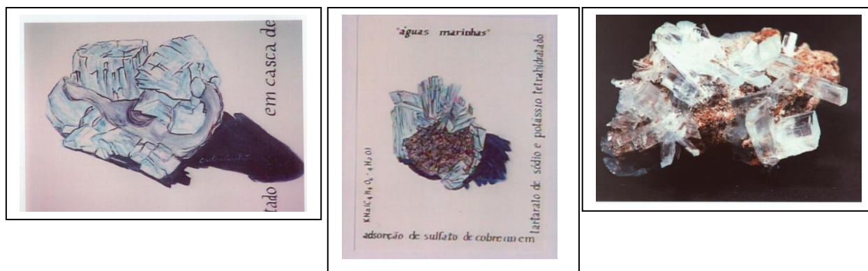
Figure 6- Potassium sodium tartrate \text{KNa(C}_4\text{H}_4\text{O}_6) \cdot 4\text{H}_2\text{O} modified by \text{Cu(II)} ions: a few drops of copper sulfate (aq) are added to the solution. Left: crystals grown on shells or “basic” hosts (calcium carbonates: marble, limestone, etc.) are more “tabular” than those of the pure compound. Right and center: on basalt crystals grow like columns. Drawings made by Cristina Fontoura Carvalhão.
