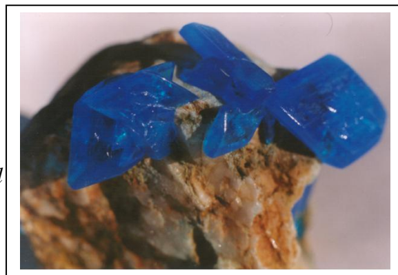
Figure1- Crystals of Copper (II) sulphate pentahydrate grown on quartz, an inert host [1]. Photographed by Cristina Fernandes (Art and Design High school teacher).
