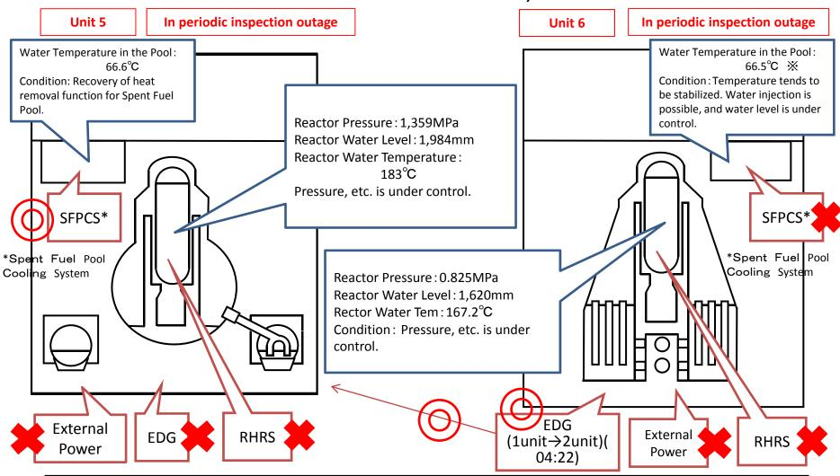
Current Conditions: Emergency Diesel Generator (1 unit →2 units (19<sup>th</sup> 04:22)) for Unit 6 is being operated. (supplying electricity to Units 5 and 6) Pump of RHR for Unit 5 started up (19<sup>th</sup> 05:00).
