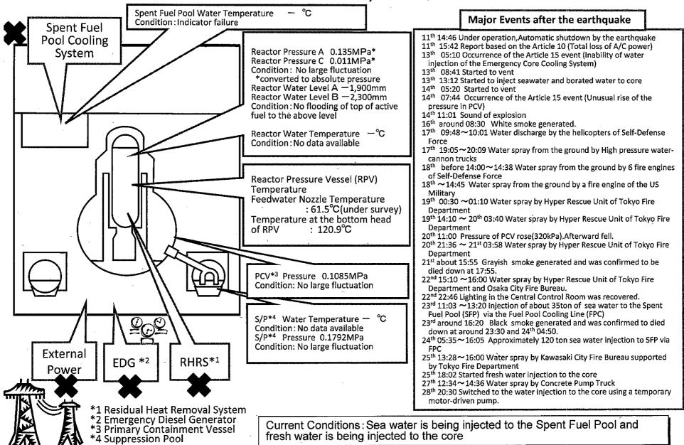
Current Conditions: Sea water is being injected to the Spent Fuel Pool and fresh water is being injected to the core
