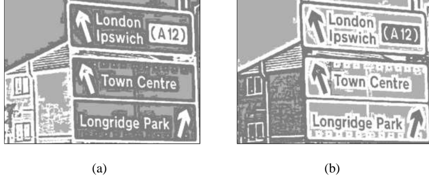
Figure 6: (a) Toggle segmentation of the positive image into background (dark gray), foreground (white) and indeterminate (light gray) pixels. (b) Toggle segmentation of the negative image.
