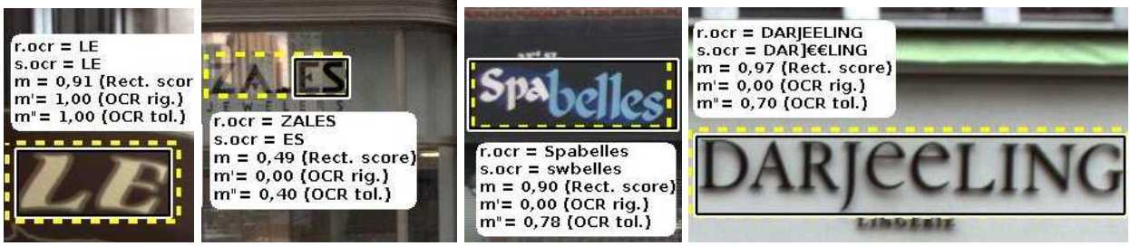
Figure 16: The OCR similarity scores m'(r, s) and m''(r, s) for \star [ check names r, s ] various text regions r extracted by SNOOPERTEXT+TESSBACK (solid outlines), and the best-matching regions s from the human-produced reference file (dashed).
