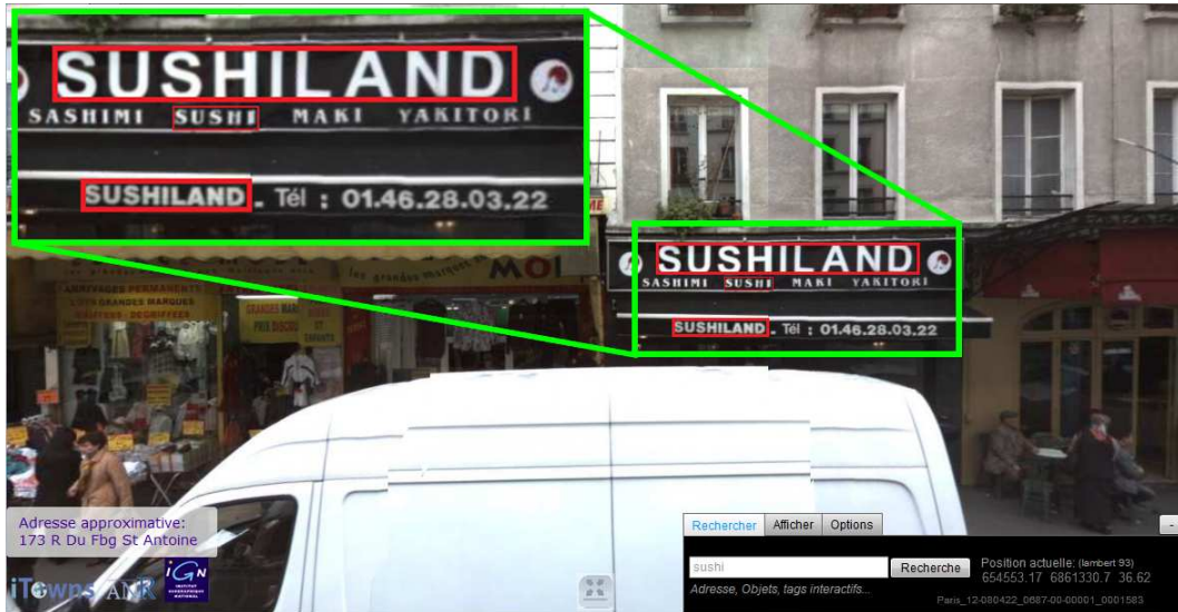
Figure 2: Result of a search for the query string “sushi” through the iTowns user interface. The textual information was extracted with our text detection system.
