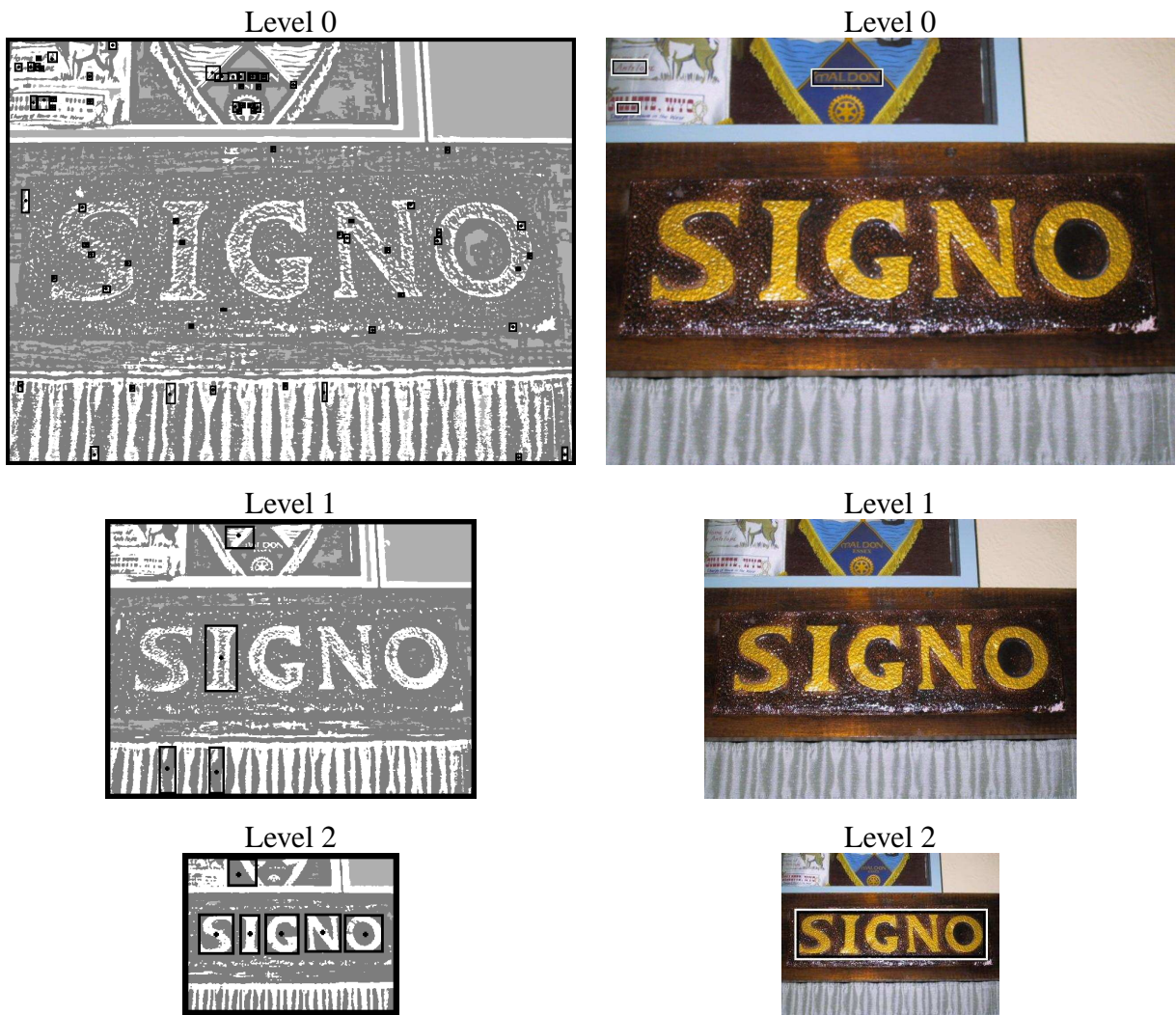
Figure 12: Example of multiscale segmentation and letter detection, illustrating texture suppression at the proper scale. Note that the letters of 'SIGNO' are oversegmented in levels 0 and 1 but correctly segmented and recognized (black boxes) in level 2.
