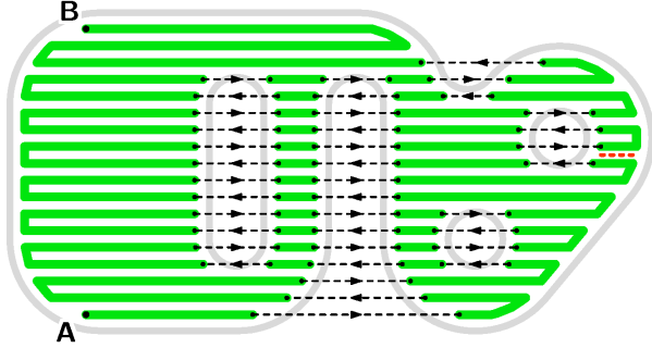
Figure 8. An alternating scan-line-order tool-path for the solid raster fill data of Figures 5 and 6. Its fab-time is 17.95 s, including 11.02 s of extrusion, and 6.93 s of air time. The red dashed line at upper right is the contact with largest cooling time, 2.25 s.
