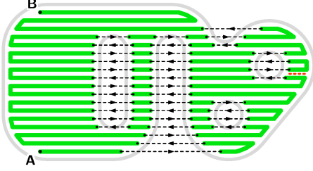
Figure 8. An alternating scan-line-order tool-path for the solid raster fill data of Figures 5 and 6. Its fab-time is 17.95 s, including 11.02 s of extrusion, and 6.93 s of air time. The red dashed line at upper right is the contact with largest cooling time, 2.25 s.
